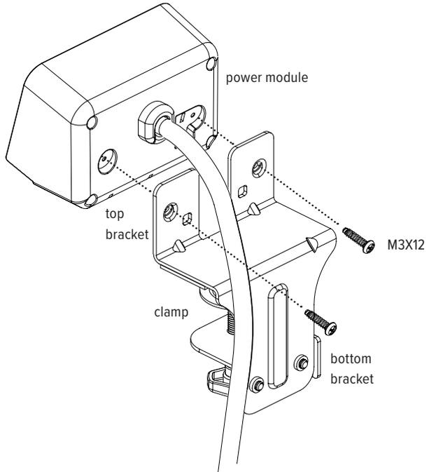
**Step #2: clamp assembled FlexCharge3 to worksurface**
